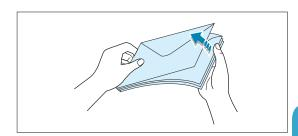
2 Load the envelopes into the input tray with the flap side down.
